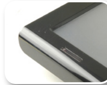
Ambient Light Sensor (Only for AFL-W19A Series)
