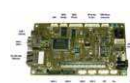
nanoETExpress Human Machine Interface (HMI) Baseboard
