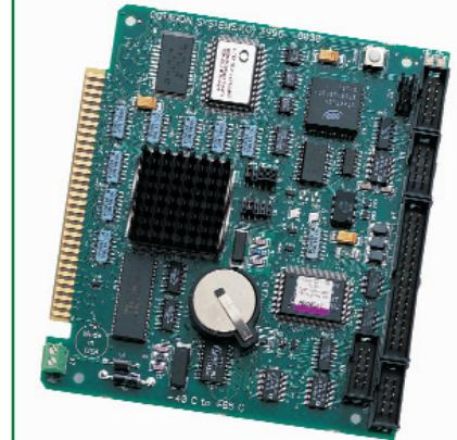
*Octagon products are designed and manufactured under the supervision of an ISO 9001-2000 certified quality management system. The 6030 will withstand high shock and vibration, and operates in temperature ranges from -40° to +85° C.*
