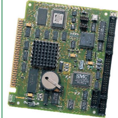
*Octagon products are designed and manufactured under the supervision of an ISO 9001-2000 certified quality management system. The 6050 will withstand high shock and vibration, and operates in temperature ranges from -40° to +85° C. This rugged single board computer will provide years of reliable service in the most challenging environments.*
