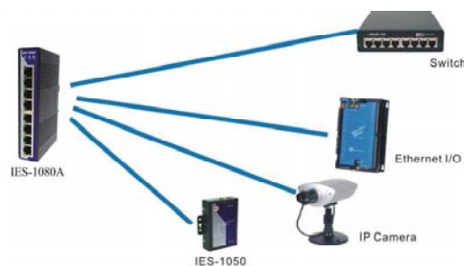
Connections of Ethernet devices
