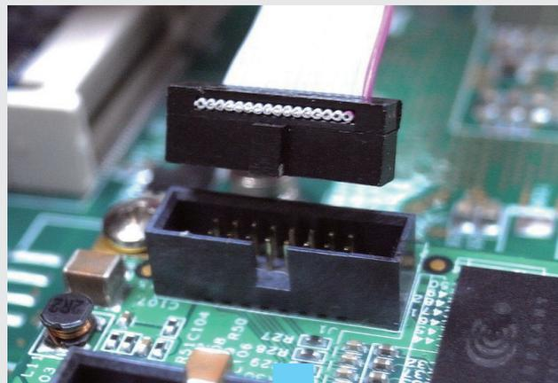
Connect 16 pin to D-sub 15 Cable for source input. Detailed pin definition please refer to 2.1 section.
